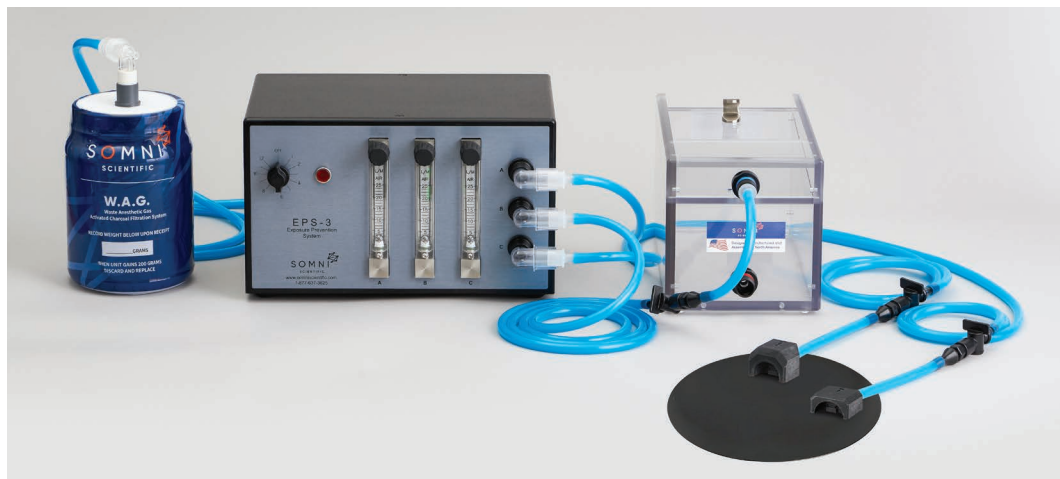
EPS-3 shown here with 3 anesthetic supply accessories connected (1 Chamber, 2 nosecones)
